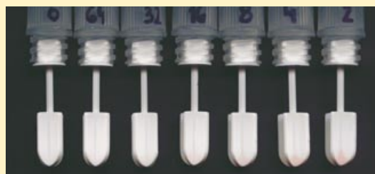
Dipstick method. Calibration curve for Lm . From left: 0, 0.23, 0.45, 0.9, 1.8, 3.6, 7.2 c (CFU/ml) \times 10^8 (coloration is dependent on concentration).
